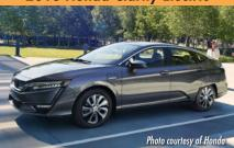
Type: Battery electric vehicle; Sedan EPA electric range: 89 miles Charging time: 3 hours @ 240V; Fast-charging capable
